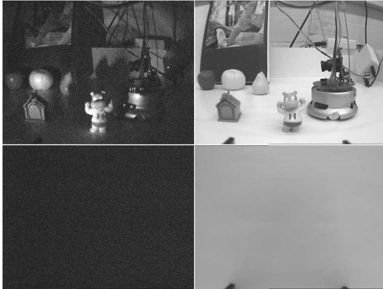
Figure 10: The 4 types of images used. All images had size 768 times 576 pixels. Note that the images taken in the dark (left) have increased noise.
