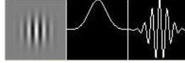
Figure 11: the smallest-size Gabor filter used. Left: standardized surface plot. Middle: standardized vertical cut. Right: standardized horizontal cut. Parameters: size: 64x64 pixels, wavelength: 8 pixels, sigma: 9.1. Maximum: 0.0438.
