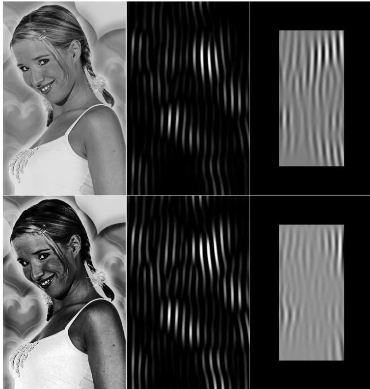
Figure 16: The difference between OpenCV's and the self-written convolution, with and without first histogram equalizing the initial picture. Top row: Left) original image. Mid) image after OpenCV's convolution. Right) image after self-written convolution. Bottom row: Left) original image after histogram equalization. Mid) image after OpenCV's convolution Right) image after self-written convolution. The filter used was the smallest Gabor. size 32 \times 32 , wavelength 8 pixels, sigma 9.1.
